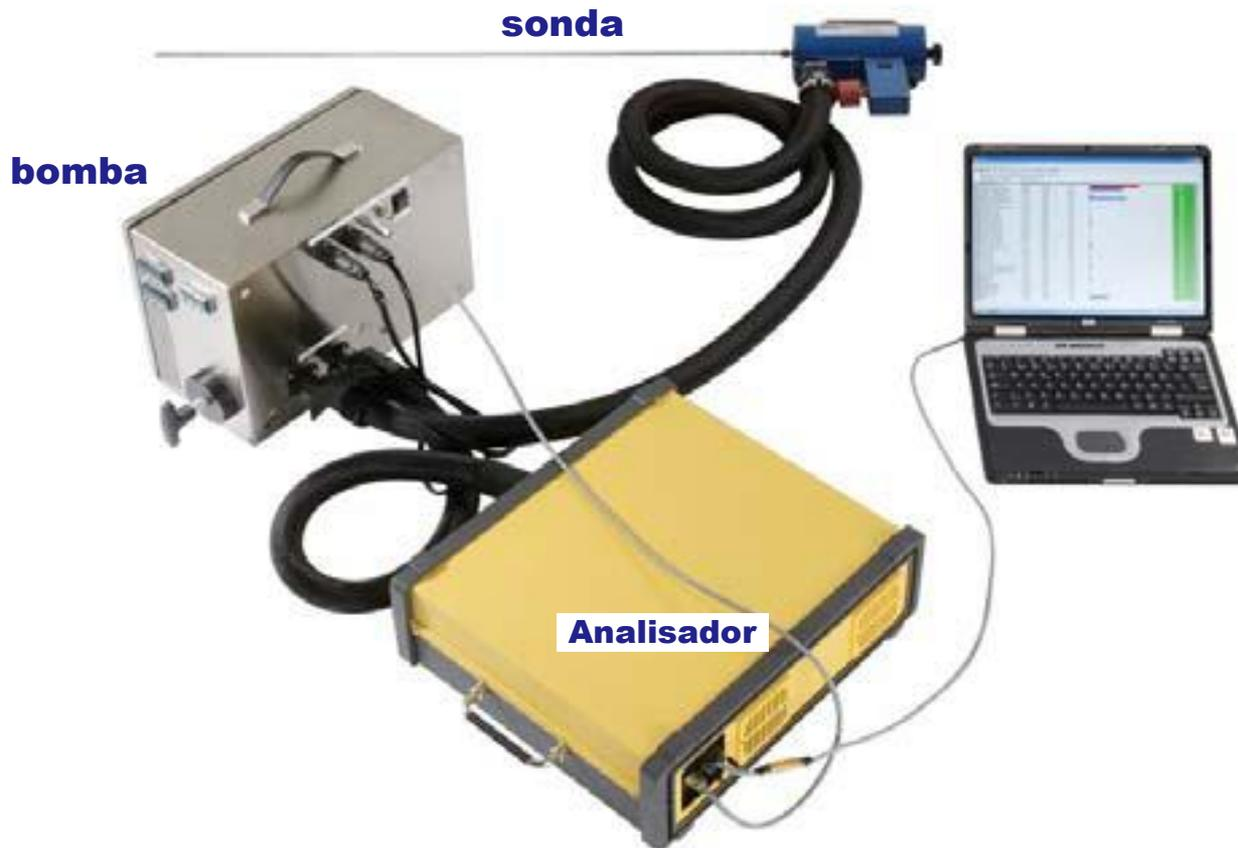
**Fourier transform infrared (FTIR) spectroscopy.**
